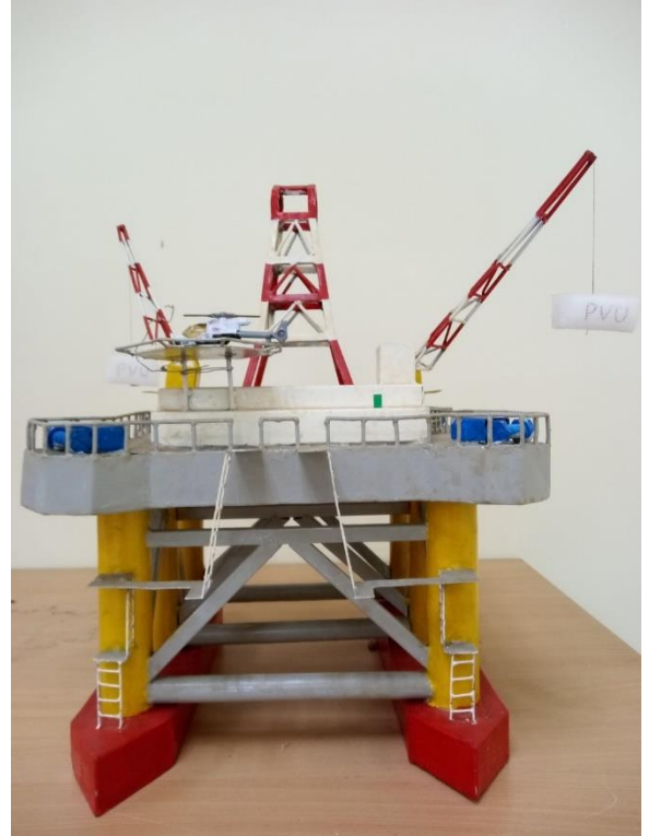
SEMI-SUBMERSIBLE Water depth: 60-3000m
