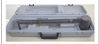
**Device: Model 140 Mud Balance** Function: Determination of fluid density
