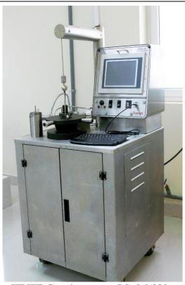
**Device: HPHT Consistometer Model 290**Function: Measure cement slurry viscosity or consistency under elevated
