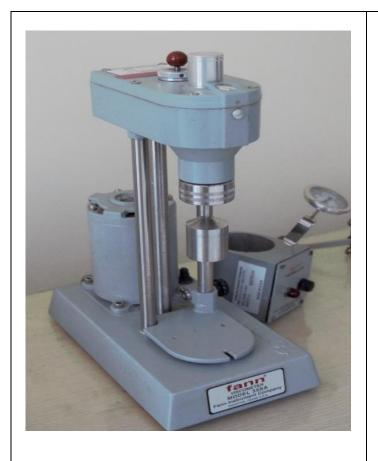
**Device: Fann 35SA viscometer** Function: Measure drilling fluid viscosity
