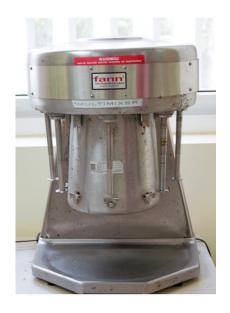
**Device: Multi-Mixer® Model 9B**Function: Mixing of drilling fluids in preparation for laboratory tests of mud materials
