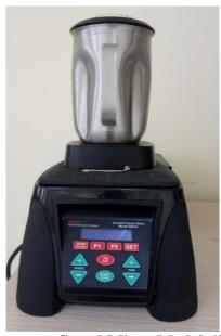
**Device: Constant Speed Mixer Model 686CS**Function: Mix cements to comply with American Petroleum Institute (API) Spec 10A
