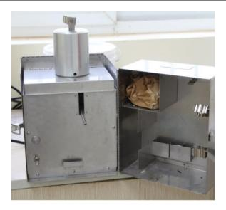
**Device: Retort 10ml Oil and Water Kit Model 871**Function: determine the quantity of liquids and solids in a drilling fluid
