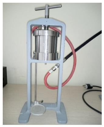
**Device: Low Temperature (LPLT) Filter Presses**Function: Determining the filtration properties of drilling muds and cement slurries
