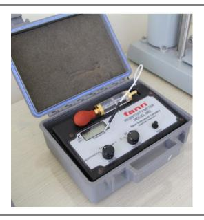
**Device: Resistivity Meter Model 88C** Function: Measure drilling fluid resistivity
